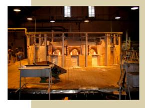
The pot furnace is the type of furnace mostly used for table ware and art glass. Mainly used for melting lead crystal glass.
